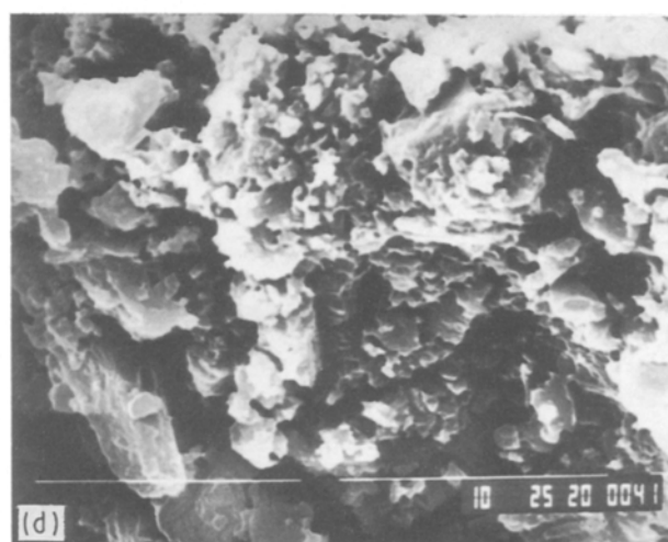
Figure 3 Scanning electron micrographs of Mg_{1.0}-V_{2.0} oxide system calcined at different temperatures for 5 h. T_c = 500^\circ C : (a) \times 350 , (b) \times 10000 . T_c = 700^\circ C : (c) \times 1500 , (d) \times 5000 . T_c = 1000^\circ C : (e) \times 5000 .
